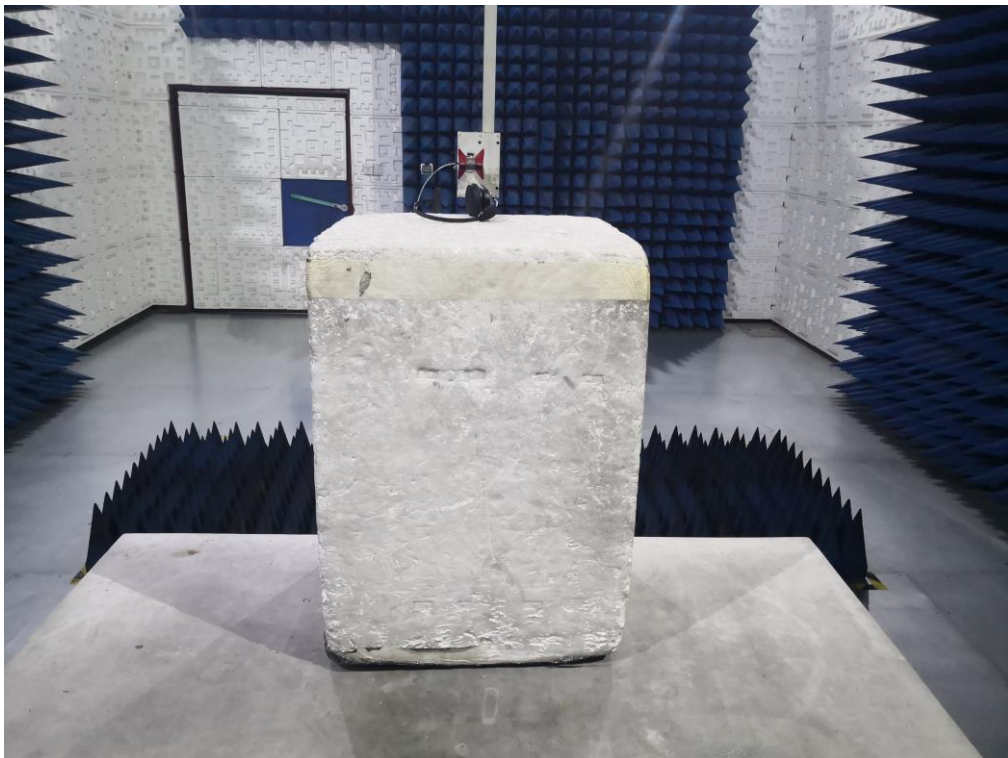
RADIATED EMISSION TEST SETUP ABOVE 1GHz
