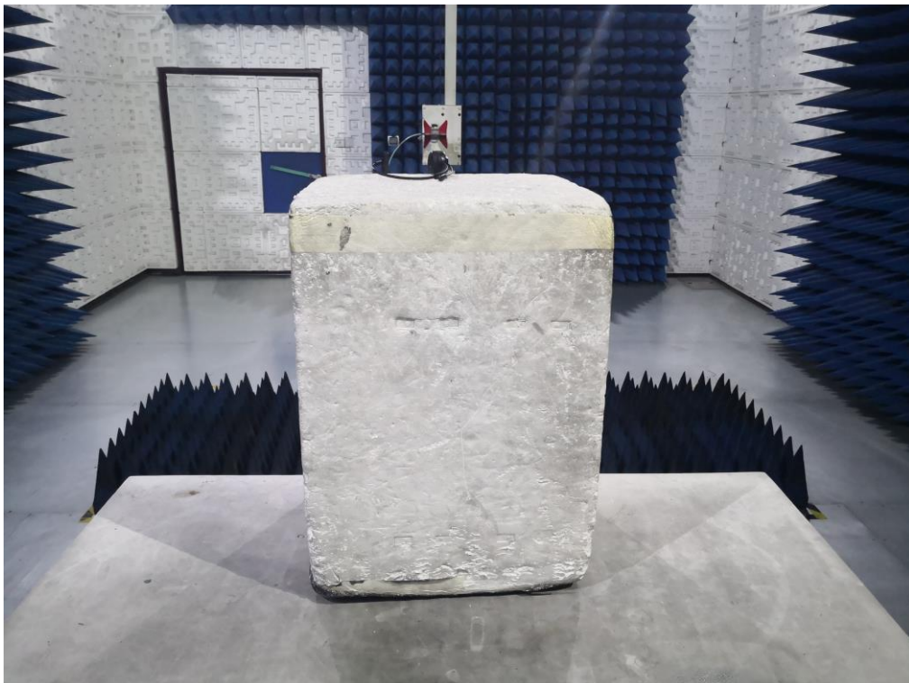
RADIATED EMISSION TEST SETUP ABOVE 1GHz
