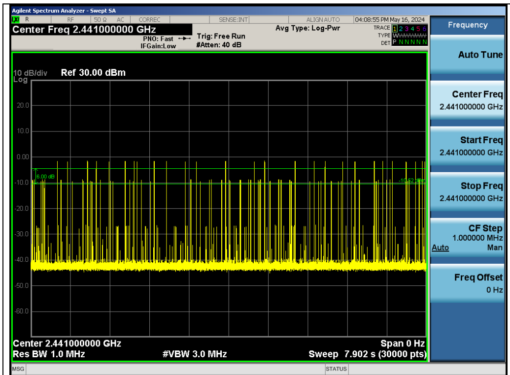
Test_Graph_EDR_HOP_ANT1_NA_3Mbps_2441_Number of Burst
