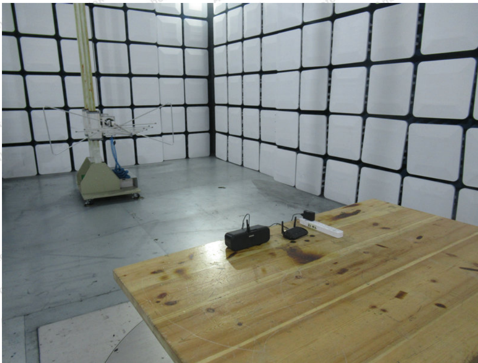
Photo of Radiation Emission Test
