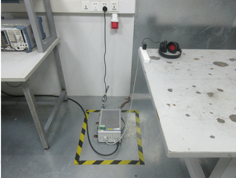
Photo of Conducted Emission Measurement
