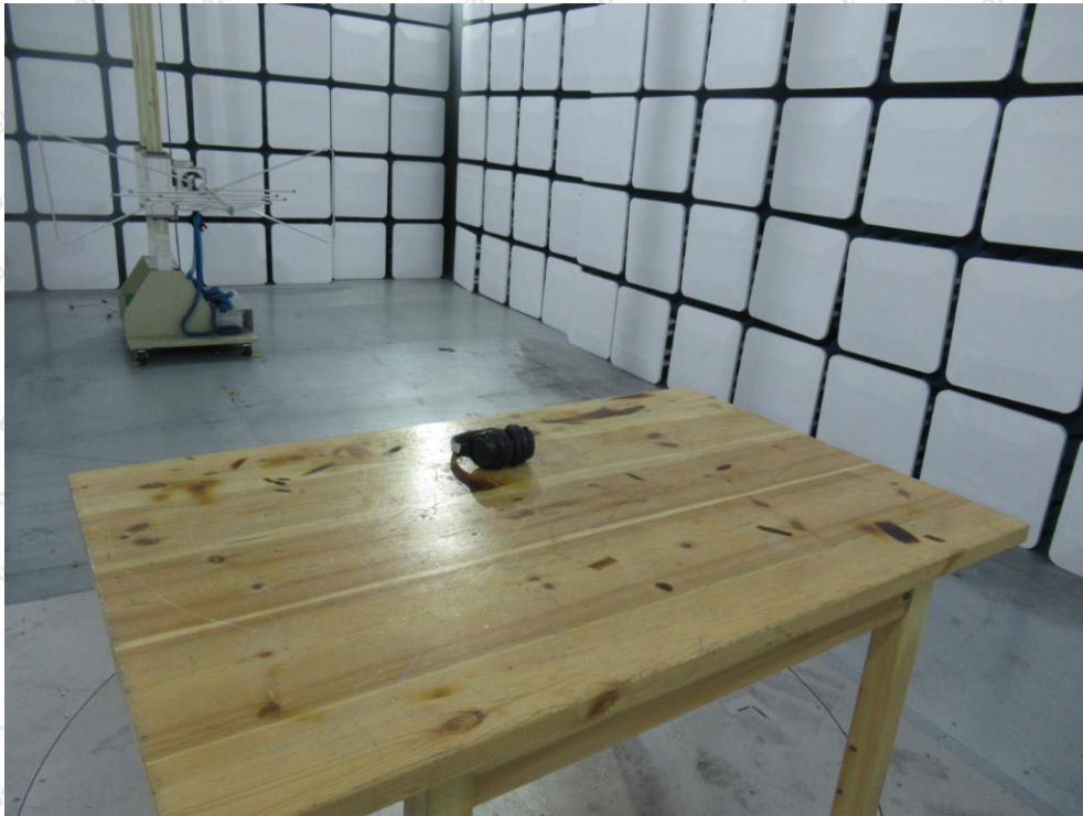
Photo of Radiation Emission Test
