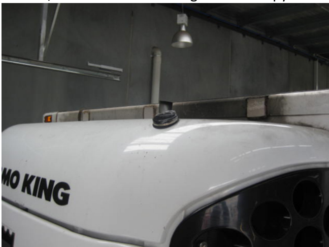
GSM/GPS Antenna Installed – side shot
