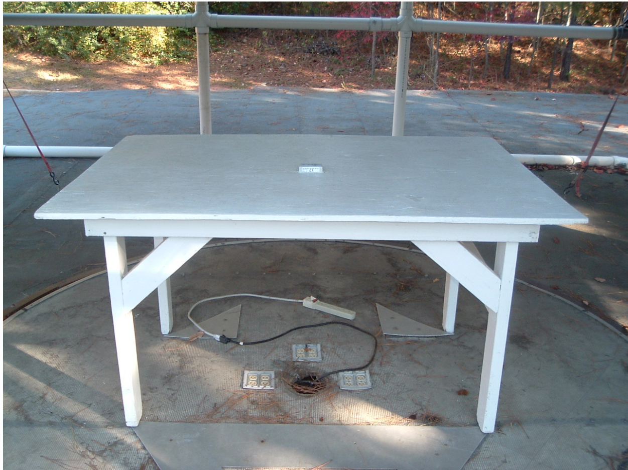
Figure 2. Photograph of Test Setup for Spurious and Fundamental Emissions Measurement, (Front View)
