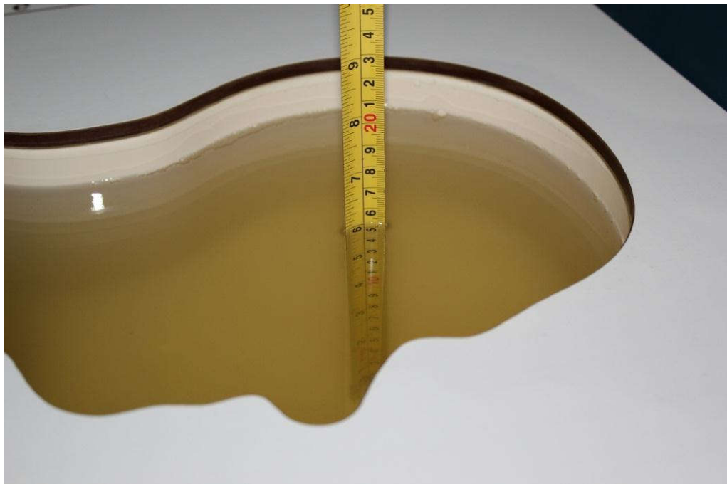
Picture 7-4: Liquid depth in the Head Phantom(2550MHz)
