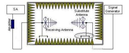
In the chamber, a substitution antenna for the frequency band of interest is placed at the reference point of the chamber. An RF Signal source for the frequency band of interest is connected to the substitution antenna with a cable that has been constructed to not interfere with the radiation pattern of the antenna. A power ( $P_{\text{Mea}}$ ) is applied to the input of the substitution antenna, and adjust the level of the signal generator output until the value of the
