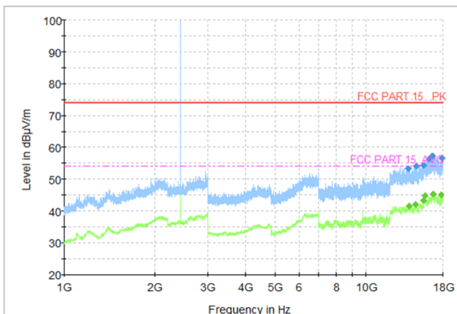
Fig. 48 Radiated Spurious Emission ( \pi/4 DQPSK, Ch39, 1 GHz ~ 18 GHz)
