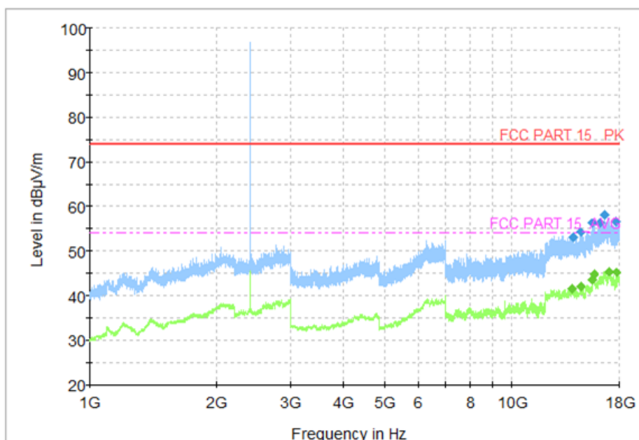
Fig. 52 Radiated Spurious Emission (8DPSK, Ch0, 1 GHz ~ 18 GHz)
