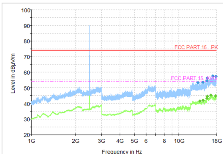
Fig. 44 Radiated Spurious Emission (GFSK, Ch78, 1 GHz ~ 18 GHz)
