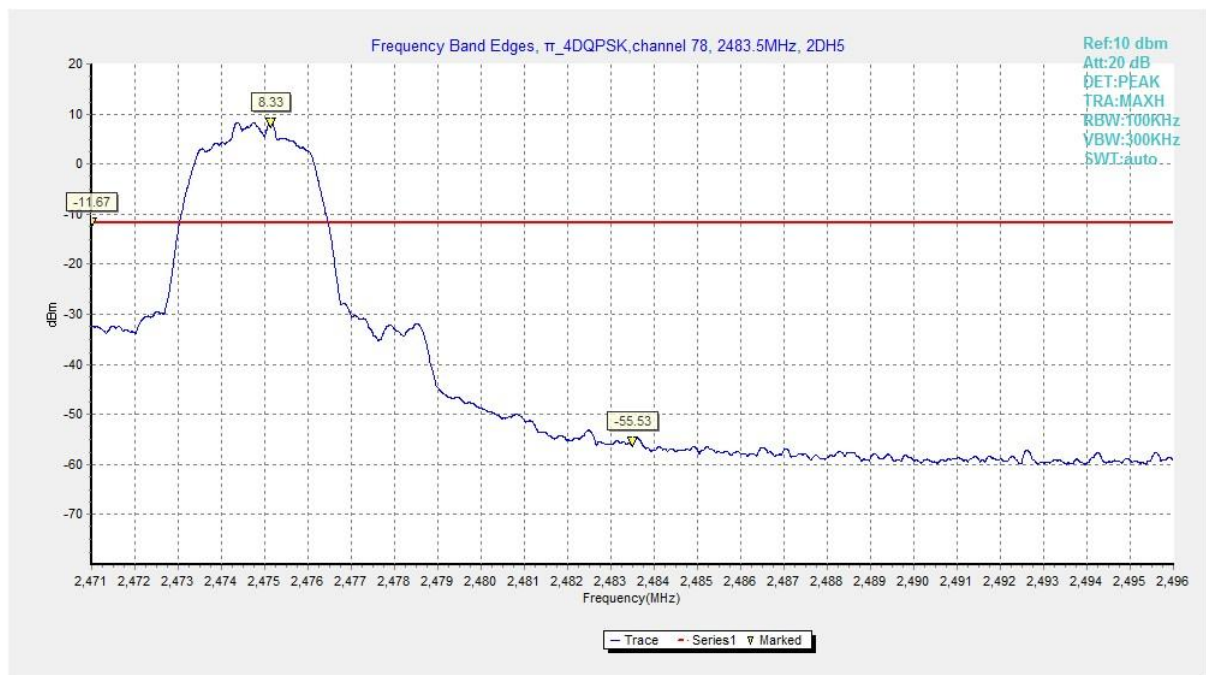
Fig. 10 Band Edges ( \pi /4 DQPSK, Ch 78, Hopping OFF)
