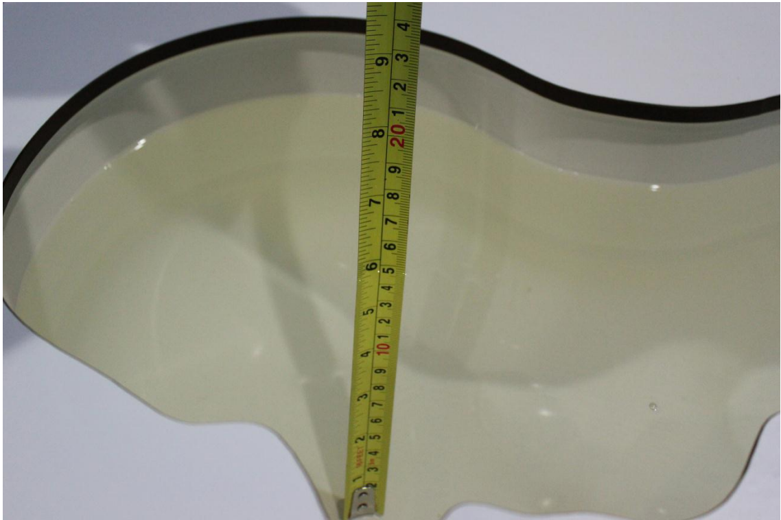
Picture 7-9: Liquid depth in the Head Phantom(5G)
