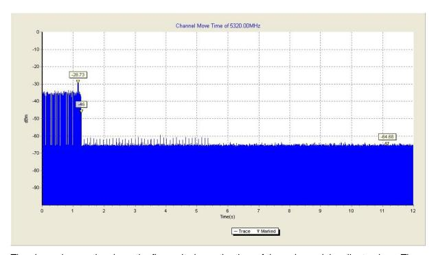
The channel move time is as the figure. It shows the time of the radar and the client pulses. The figure shows that the client stops transmission within 10 seconds, and no transmissions occur after 10 seconds later of the radar burst signal.
