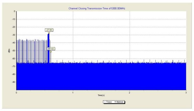
The closing transmission time is as the figure, and the result is 36ms
