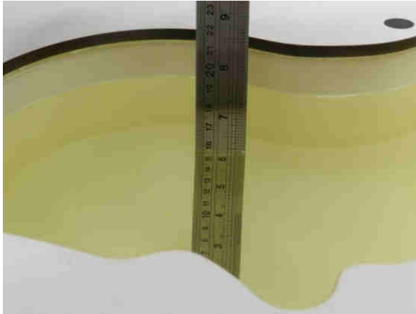
Fig 10.1 Photo of Liquid Height for Head SAR
