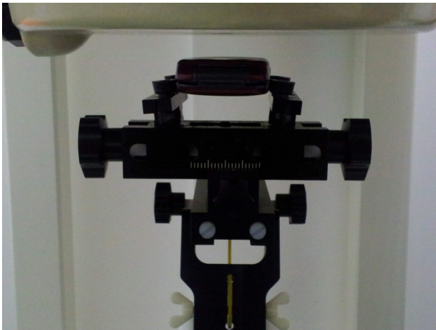
Back of the DUT with Phantom 1.5 cm Gap For Sample 2
