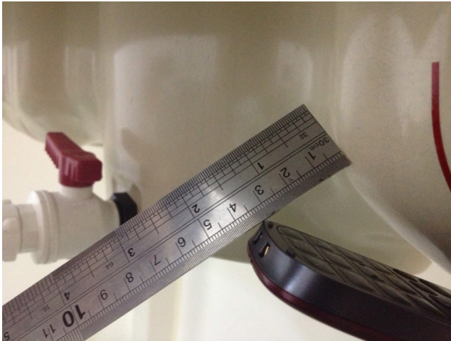
Left Cheek position - Separation distance 3.3cm between mouth and antenna For Sample 2
