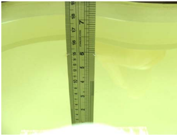
Fig 6.1 Photo of Liquid Height for Head SAR
