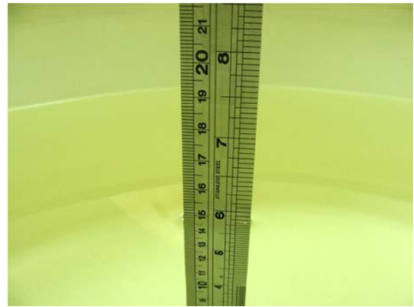
Fig 6.2 Photo of Liquid Height for Body SAR
