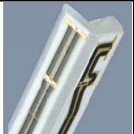
Fig 5.2 Photo of E-field Probe
