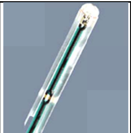
Fig 5.3 Photo of H-field Probe
