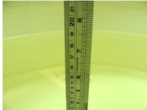
Fig 6.2 Photo of Liquid Height for Body SAR
