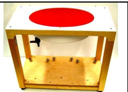
Fig 5.10 Photo of ELI4 Phantom
