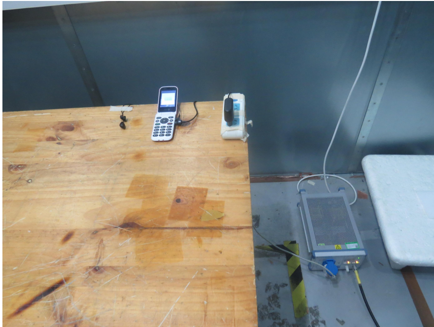
Picture 3 Conducted Emission Test Setup
