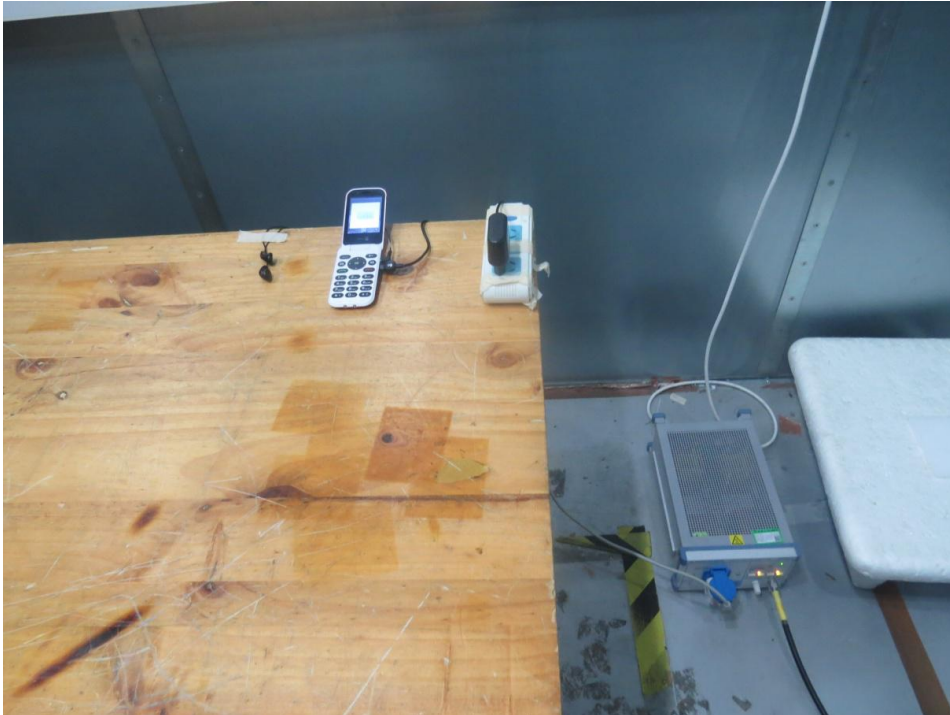
Picture 3 Conducted Emission Test Setup
