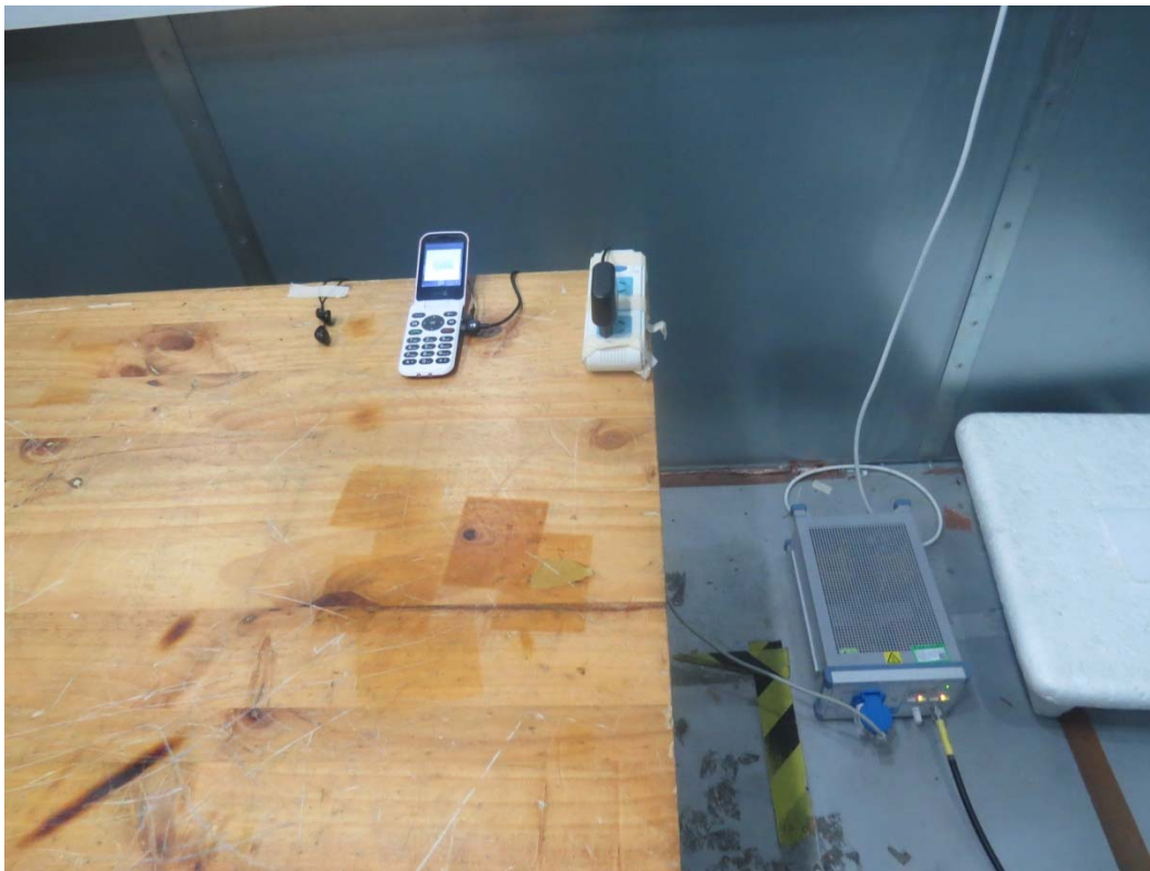
Picture 3 Conducted Emission Test Setup
