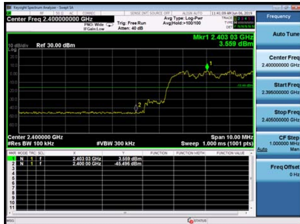
BT 3DH5 CH0, Carrier frequency (MHz): 2402
