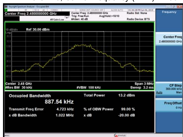
BT DH5 CH78, Carrier frequency (MHz): 2480
