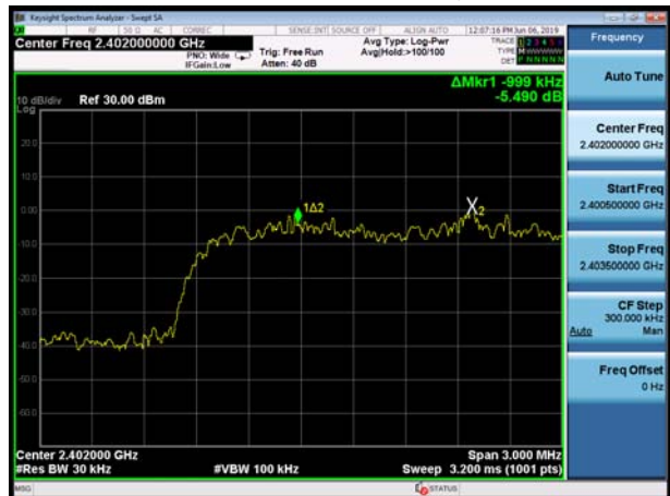
BT 2DH5 CH39, Carrier frequency (MHz): 2441
