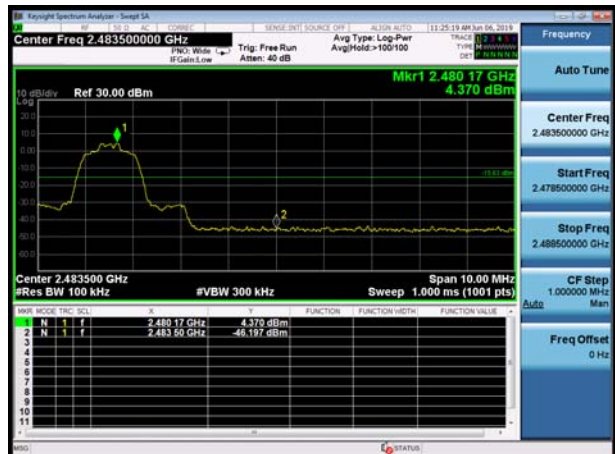
BT 3DH5 CH78, Carrier frequency (MHz): 2480
