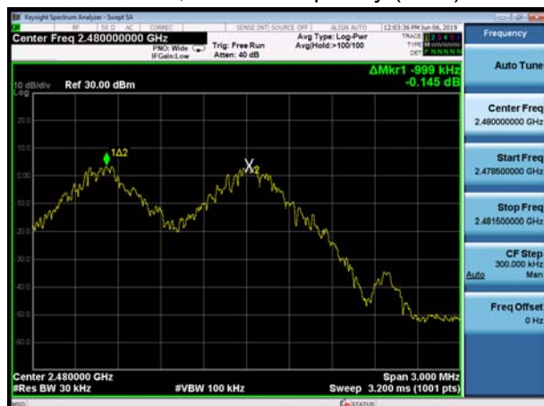
BT DH5 CH78, Carrier frequency (MHz): 2480
