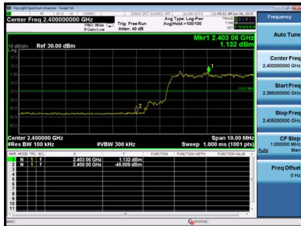
BT 3DH5 CH0, Carrier frequency (MHz): 2402
