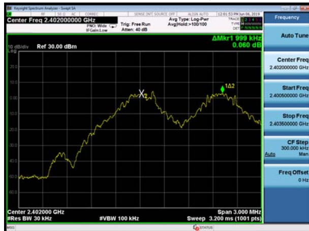
BT DH5 CH39, Carrier frequency (MHz): 2441
