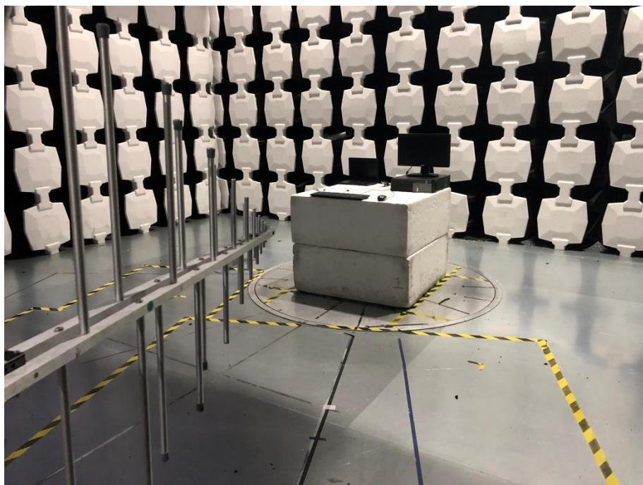
Description: Radiated Emission Test Setup
