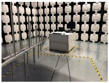
Description: Radiated Emission Test Setup
