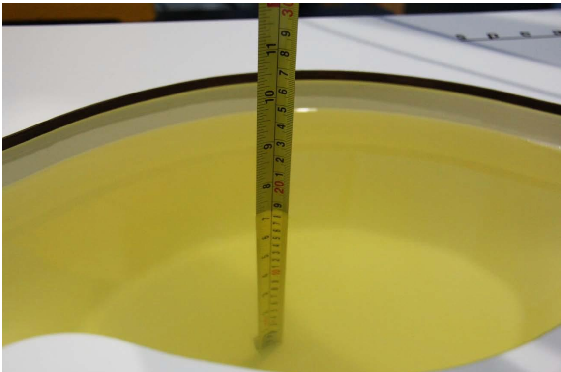
Picture 7-4: Liquid depth in the Flat Phantom(2450MHz)
