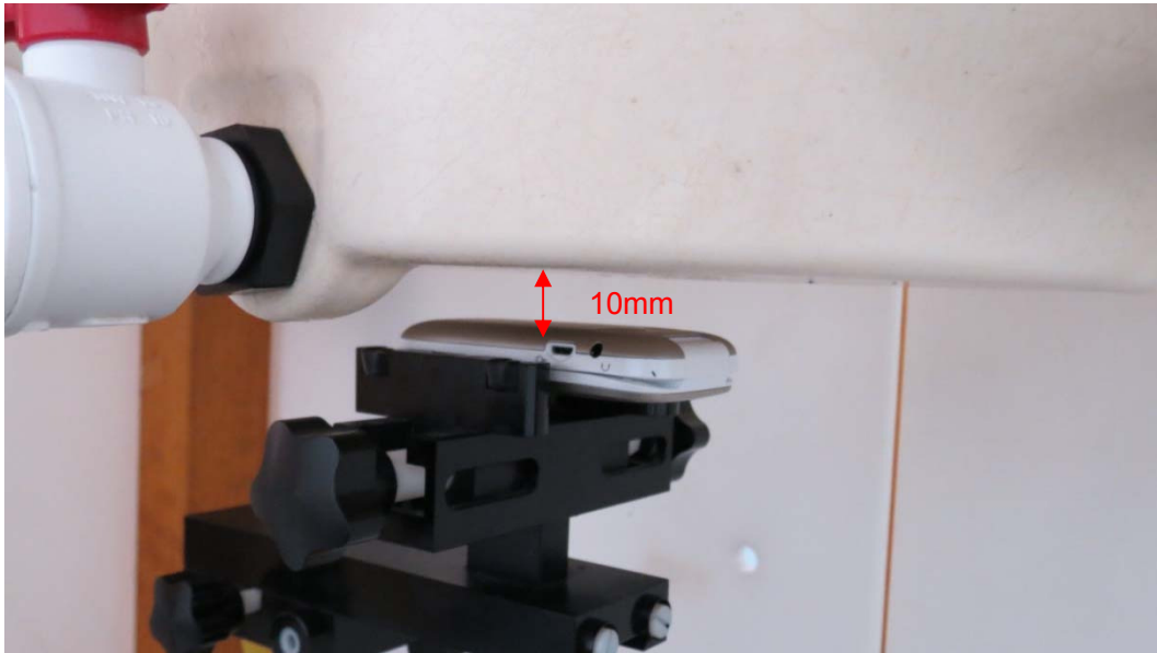
Picture 10: Back Side with closed clamshell, the distance from handset to the bottom of the Phantom is 10mm
