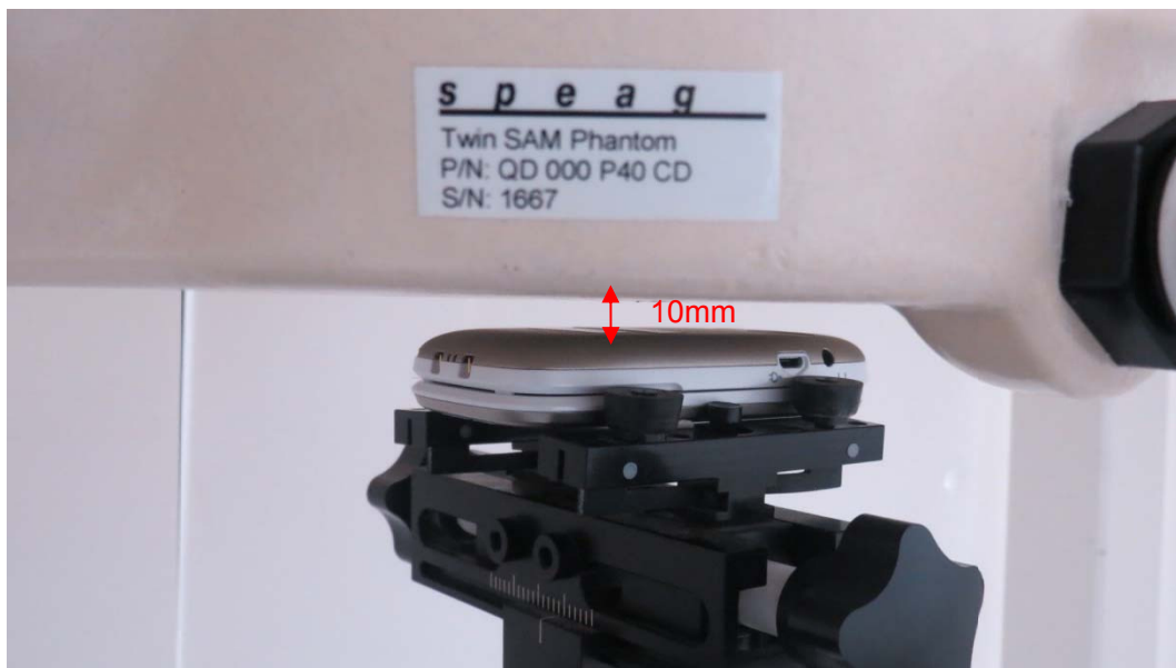
Picture 11: Front Side with closed clamshell, the distance from handset to the bottom of the Phantom is 10mm
