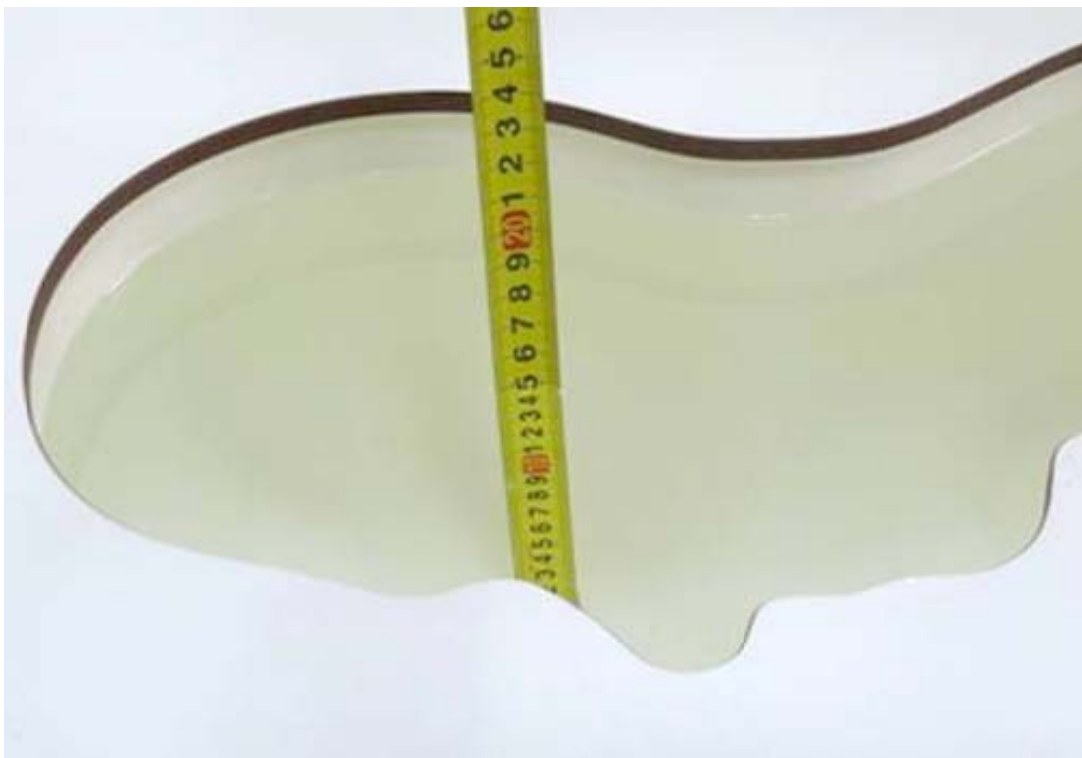
Picture 4: liquid depth in the head Phantom (1900 MHz, 15.3cm depth)
