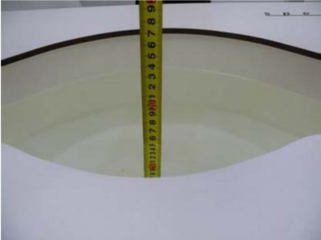
Picture 3: Liquid depth in the flat Phantom (1900 MHz, 15.2cm depth)
