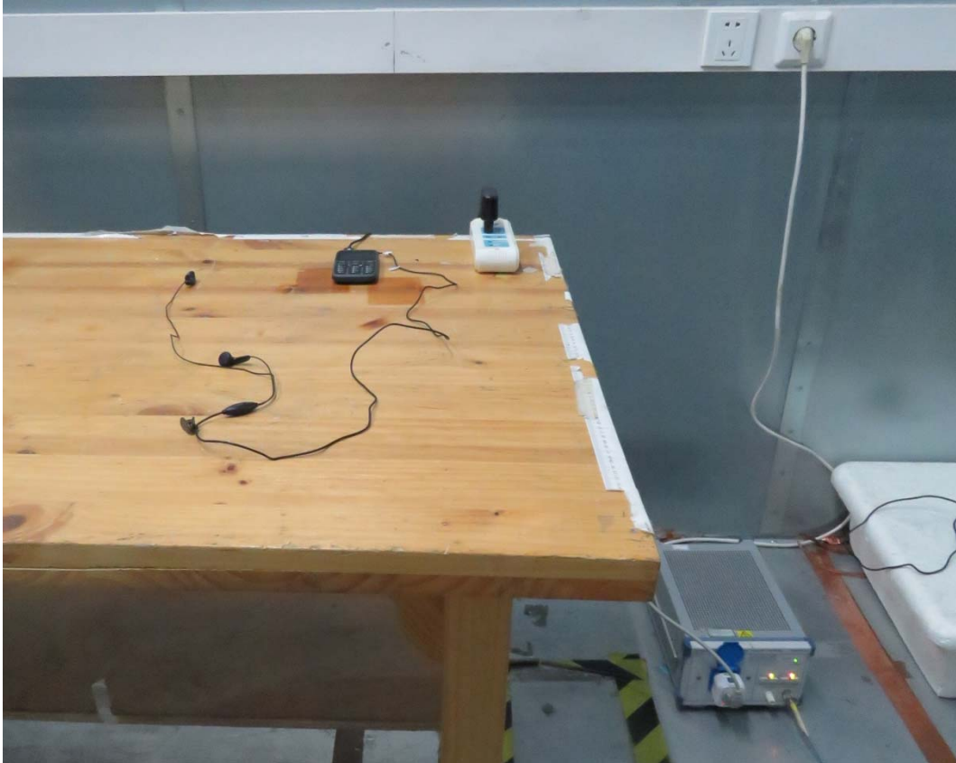
Picture 3 Conducted Emission Test Setup
