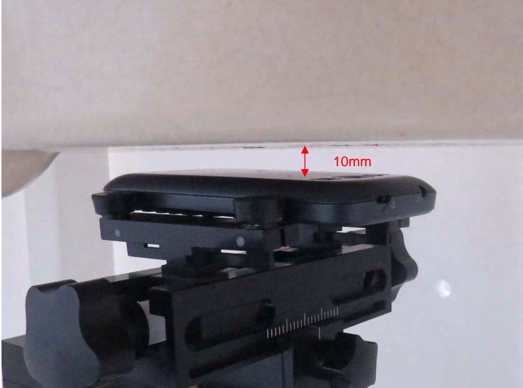
Picture 10: Back Side, the distance from handset to the bottom of the Phantom is 10mm
