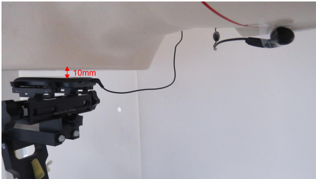
Picture 13: Back Side with Earphone 2, the distance from handset to the bottom of the Phantom is 10mm
