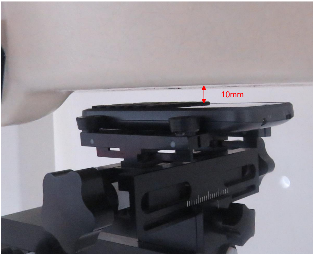
Picture 11: Front Side, the distance from handset to the bottom of the Phantom is 10mm
