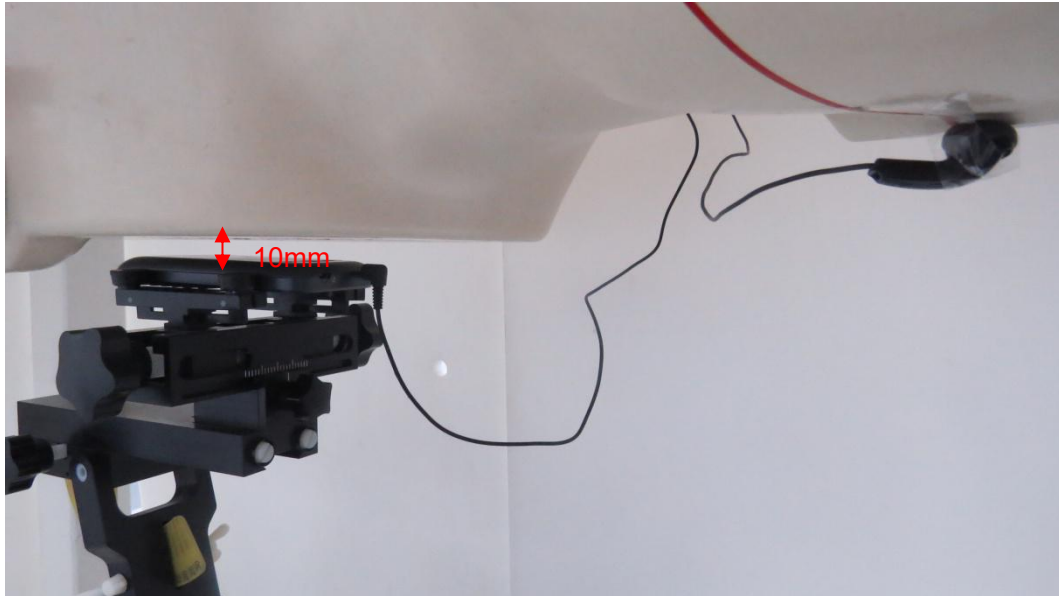
Picture 12: Back Side with Earphone 1, the distance from handset to the bottom of the Phantom is 10mm
