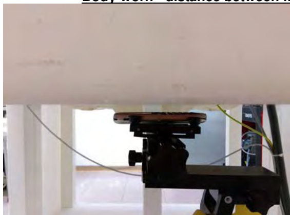
Fig.7 EUT Front side to flat phantom
