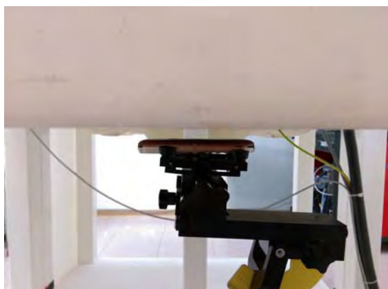
Fig.8 EUT Back side to flat phantom
