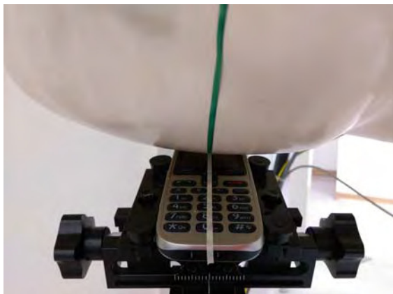
Fig.4 Right Head Section / Ear-Tilt Position(15°)
