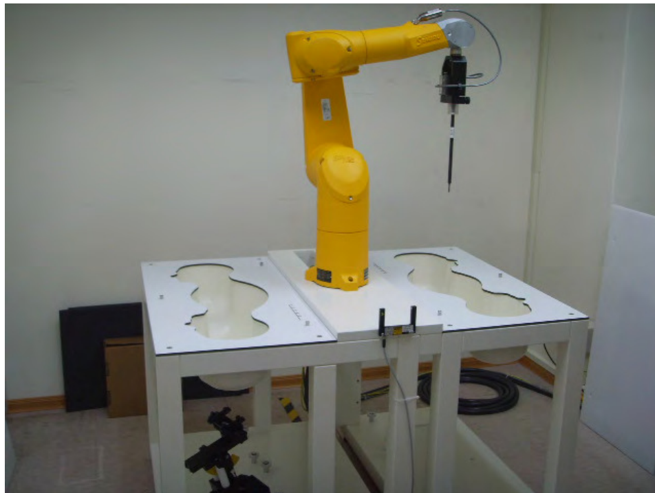
Fig.1 Photograph of the SAR measurement system
