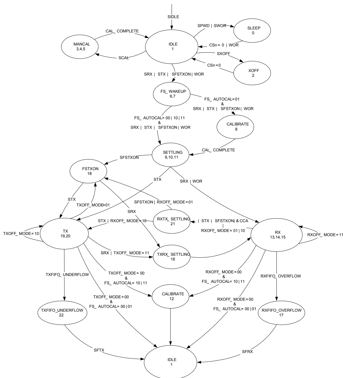
Figure 15: Complete Radio Control State Diagram
