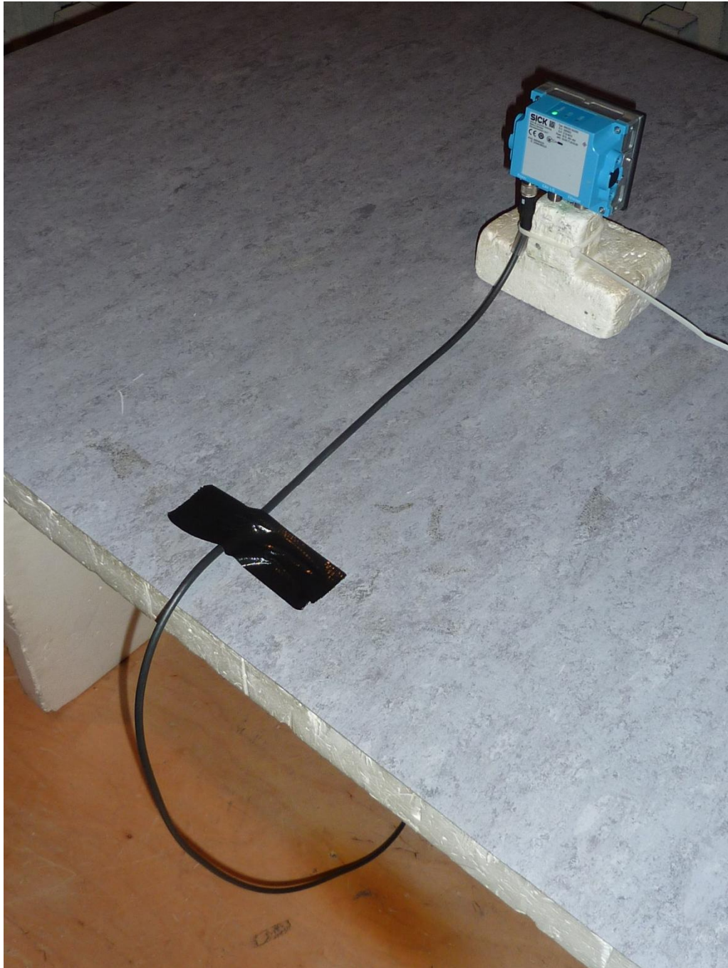
170913_ue.JPG: RMS320-343300, test setup fully anechoic chamber (table, pos. 1)
