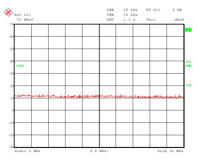
No emissions above the noise floor of the measurement system (max. 33 dB $\mu$ V/m (measured with peak detector)) found during the preliminary measurement. So no final measurements on the outdoor test site were carried out.
