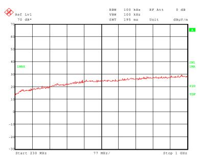
No emissions above the noise floor of the measurement system (max. 30 dB $\mu$ V/m (measured with peak detector)) found during the preliminary measurement. So no final measurements on the open area test site were carried out.
