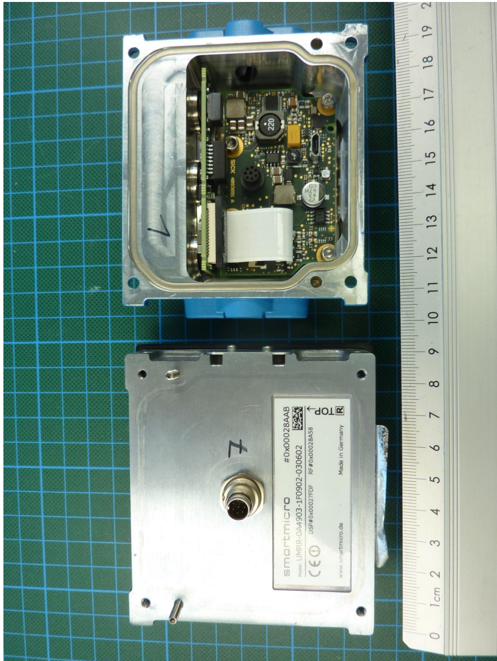
170913_5.JPG: RMS320-343300, internal view 1 (radar module removed)
