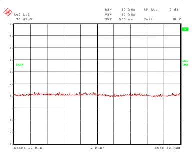
No significant frequencies above the noise floor of the system (max. 33 dB $\mu$ V/m (measured with peak detector) at 3 m distance) were found during the preliminary radiated emission test, so no measurements were carried out on the outdoor test site.
