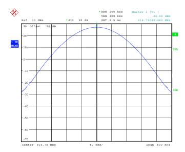
152541\_132.wmf: Maximum peak output power at the middle of the assigned frequency band, port 2:
