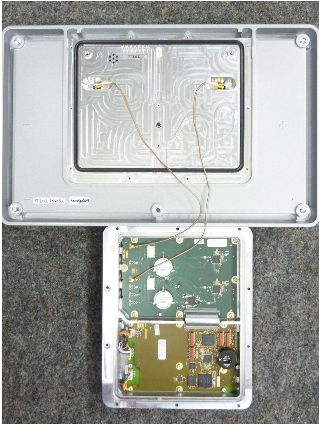
152541_1i.JPG: RFU650-10101, internal view, housing opened
