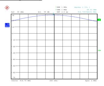
135012\_85.wmf: Maximum peak output power at the middle of the assigned frequency band (power setting 25 dBm):
