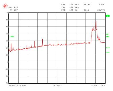
The following frequencies were found outside the restricted bands during the preliminary radiated emission test:
