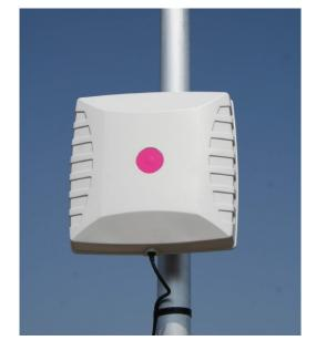
This antenna covers both EU and USA RFID bands. The antenna has been designed to be waterproof and is easy to install. It is circularly polarised for reading in any orientation. It can be used for improved indoor GSM coverage, due to circular polarisation. VSWR is typically less then 1.2:1, giving a return loss better then 20dB.
