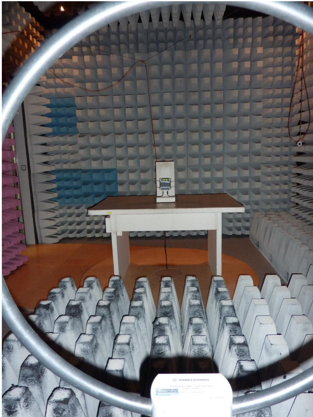
131992_10.JPG: RFU620-10101, test set-up fully anechoic chamber
