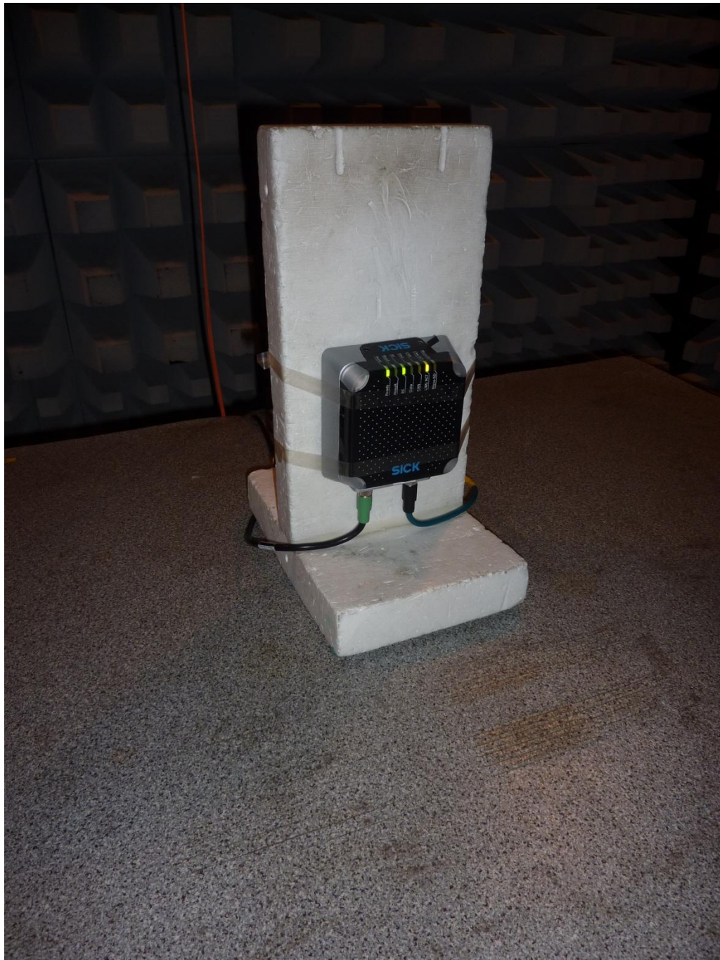
131992_7.JPG: RFU620-10101, test set-up fully anechoic chamber
