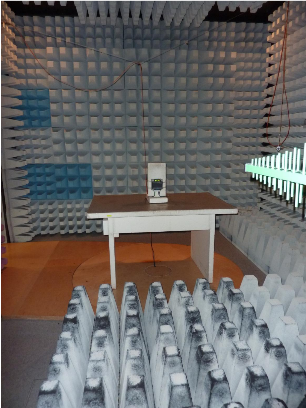
131992_8.JPG: RFU620-10101, test set-up fully anechoic chamber
