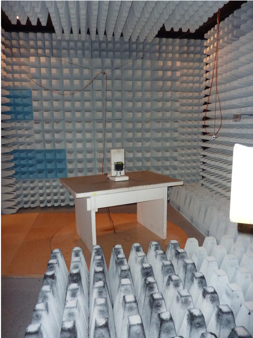
131992_9.JPG: RFU620-10101, test set-up fully anechoic chamber
