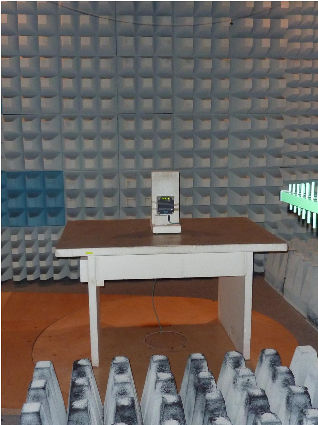
131991_3.JPG: RFU620-10501, test set-up fully anechoic chamber
