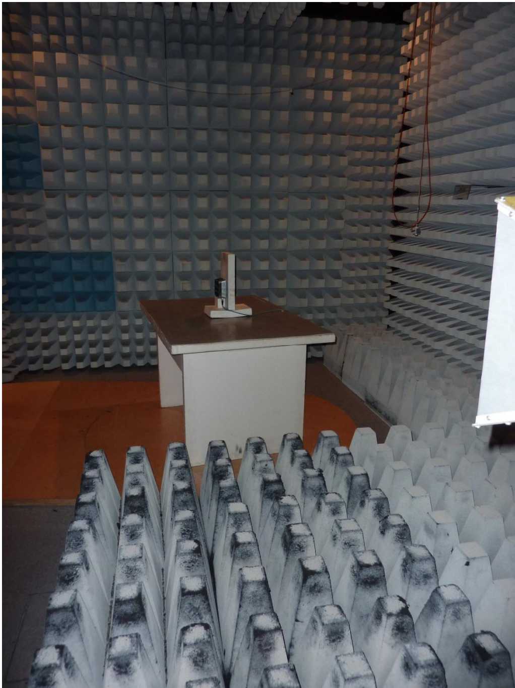
131991_4.JPG: RFU620-10501, test set-up fully anechoic chamber
