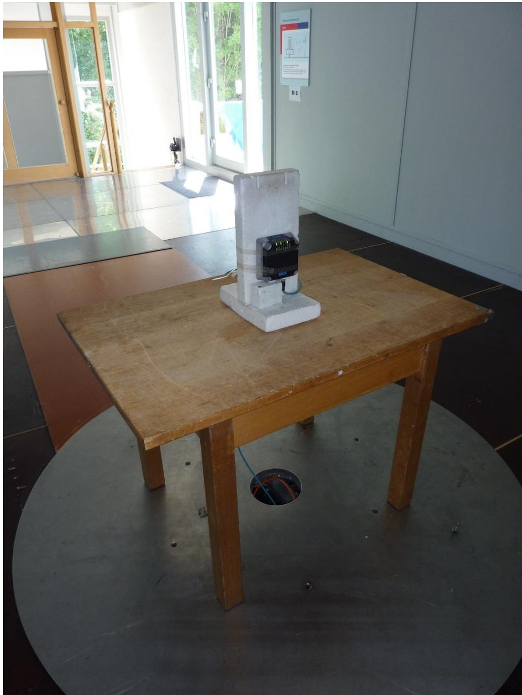
131991_6.JPG: RFU620-10501, test set-up open area test site
