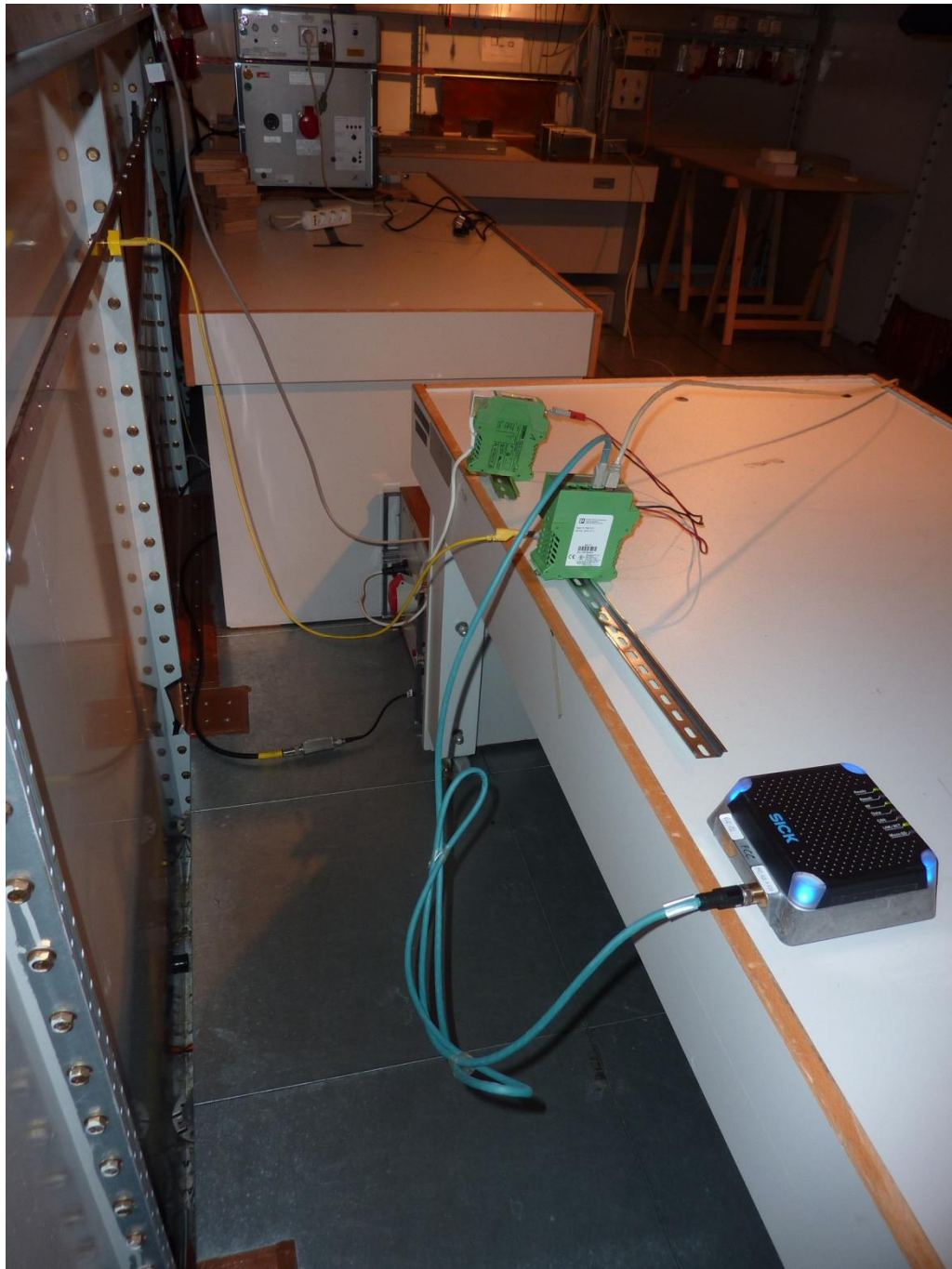
131991_7.JPG: RFU620-10501, test set-up shielded chamber
