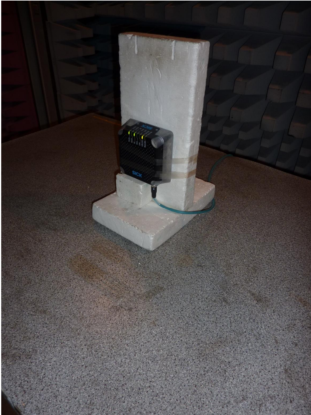
131991_2.JPG: RFU620-10501, test set-up fully anechoic chamber
