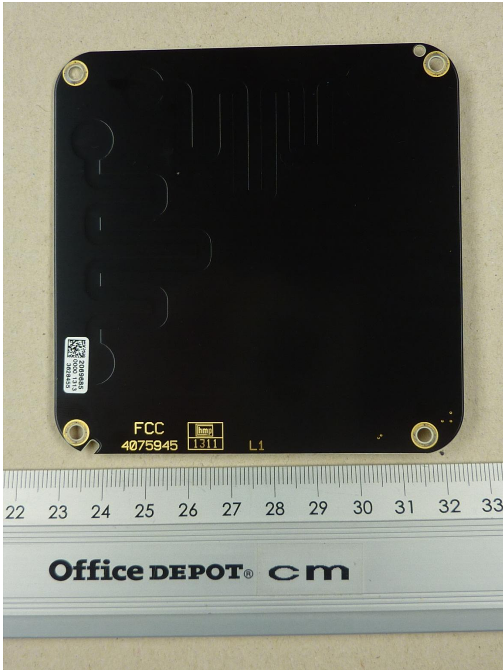
131991_h.JPG: RFU620-10501, EK-Koppler PCB, top view
