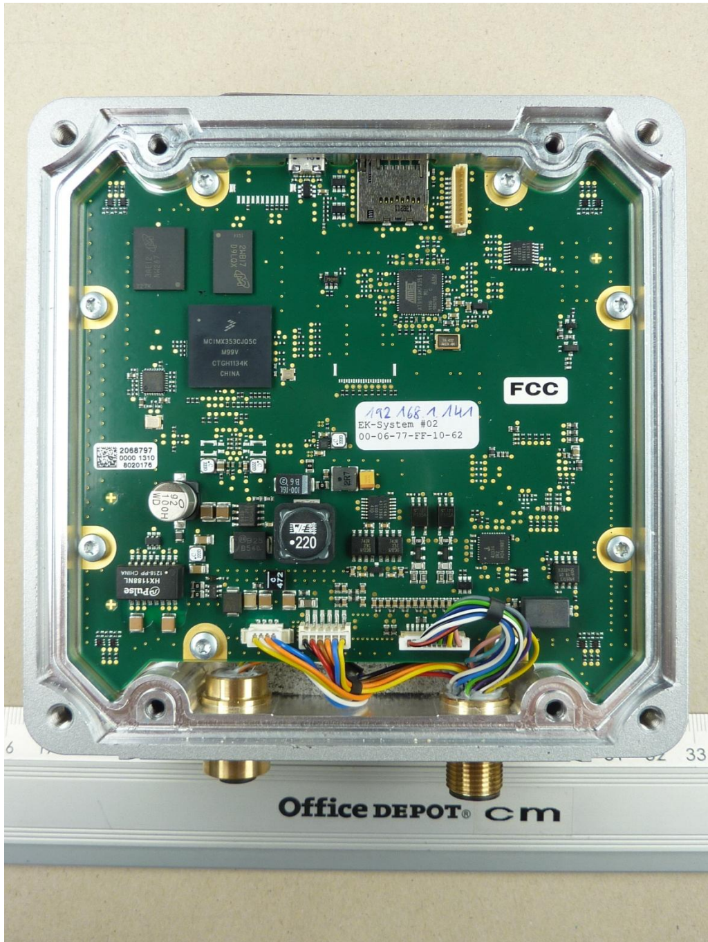
131992_c.JPG: RFU620-10101, internal view 1 (cover removed)
