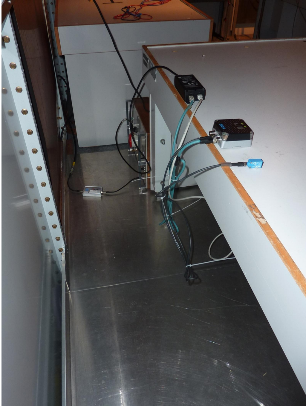
181673_20.jpg: RFU610-10601, test set-up shielded chamber
