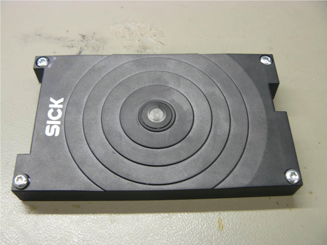
Case upper side with internal antenna
