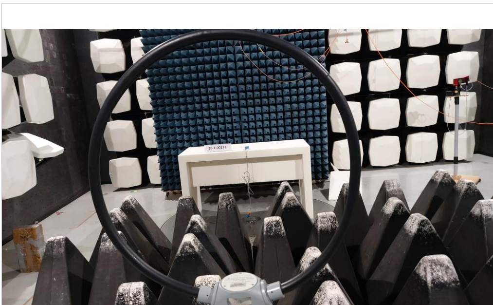
Photograph 4: EUT Setup Magnetic Field Measurements in the Semi anechoic chamber
