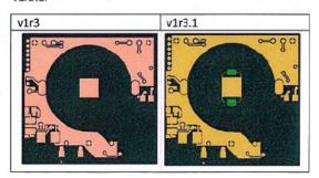
RF performance is not affected, since antennas are on top side of the PCB, which is shielded by ground plane in the inner layer from the slightly adjusted bottom layer.
