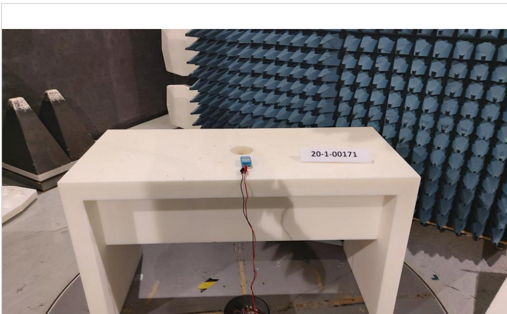
Photograph 2: EUT Test Setup in the Semi anechoic chamber, Radiated interference field
