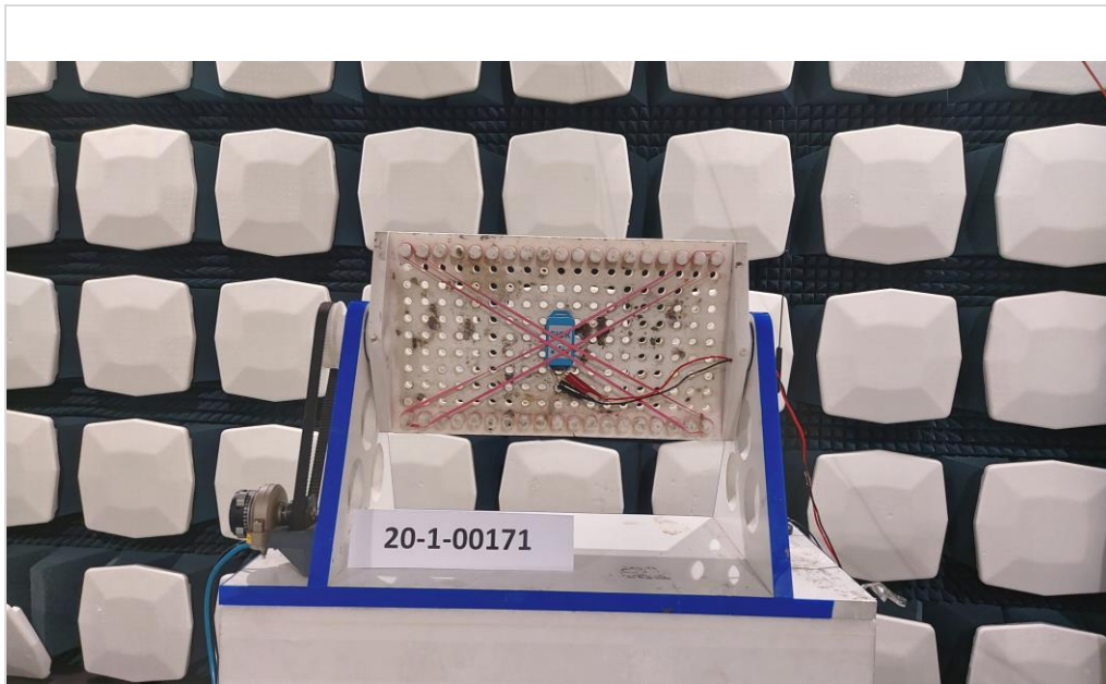
Photograph 5: EUT Test Setup in the anechoic chamber, Radiated interference field
