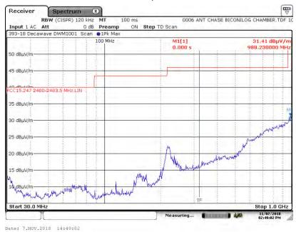
A3.2.6. Measurement Results: Z-Axis, Vertical Antenna
