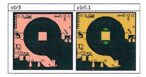
RF performance is not affected, since antennas are on top side of the PCB, which is shielded by ground plane in the inner layer from the slightly adjusted bottom layer.
