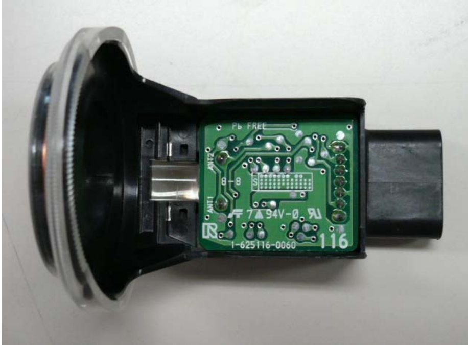
PC board inside the case
