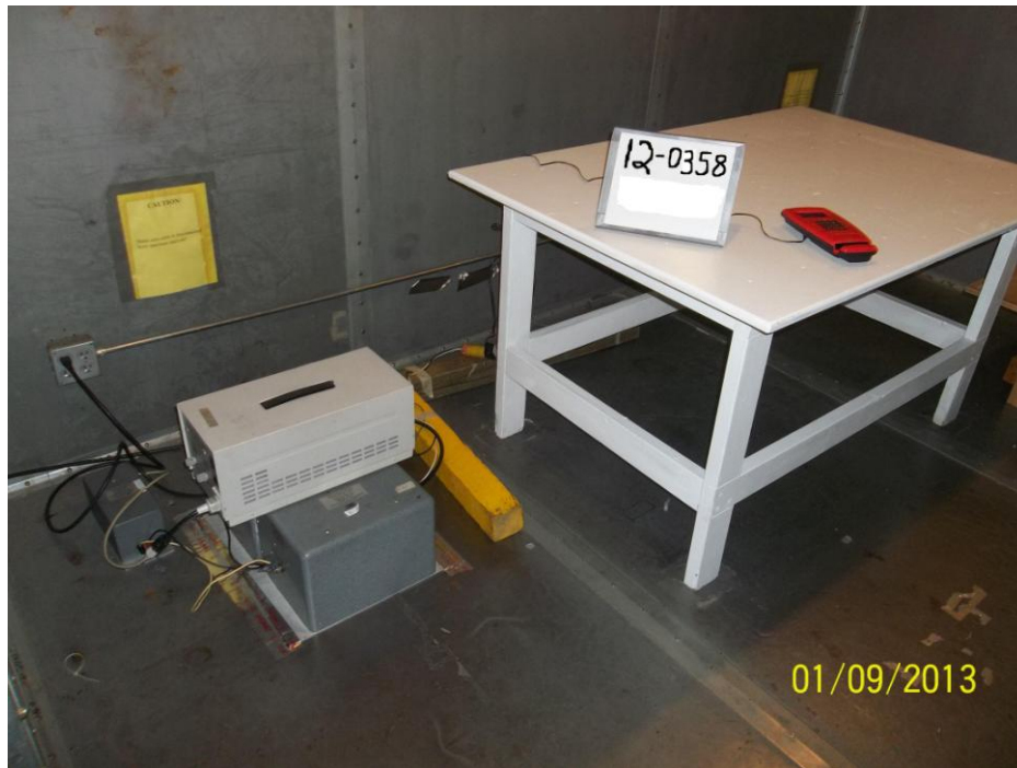
Figure 4- Test Setup Powerline Emissions
