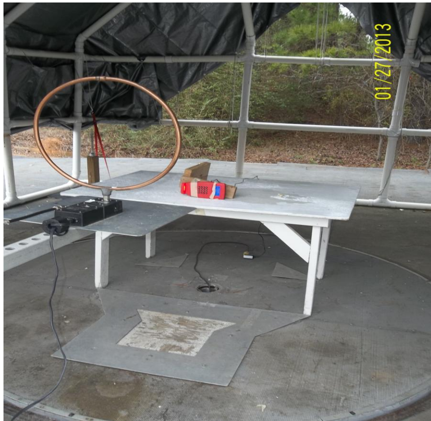
Figure 3- Test Setup Radiated Emissions Below 30 MHz
