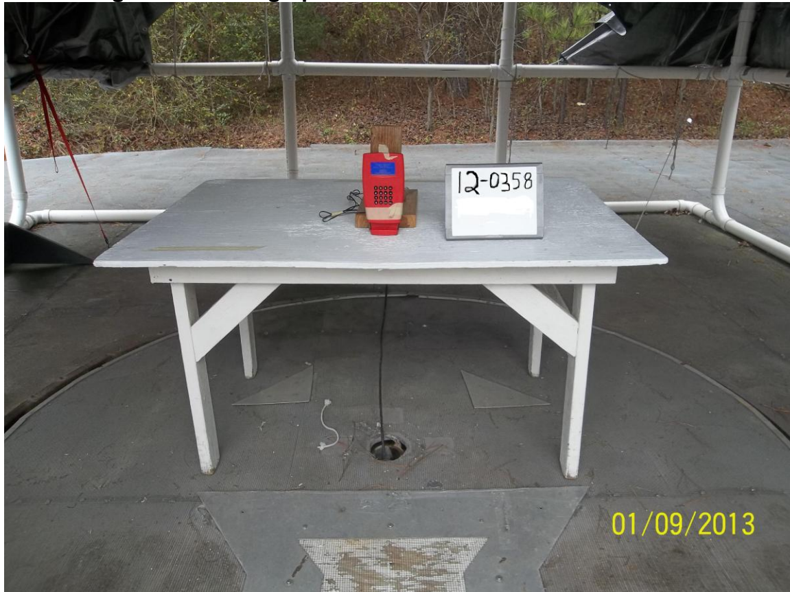
Figure 1- Test Setup Radiated Emissions 30 MHz to 1 GHz
