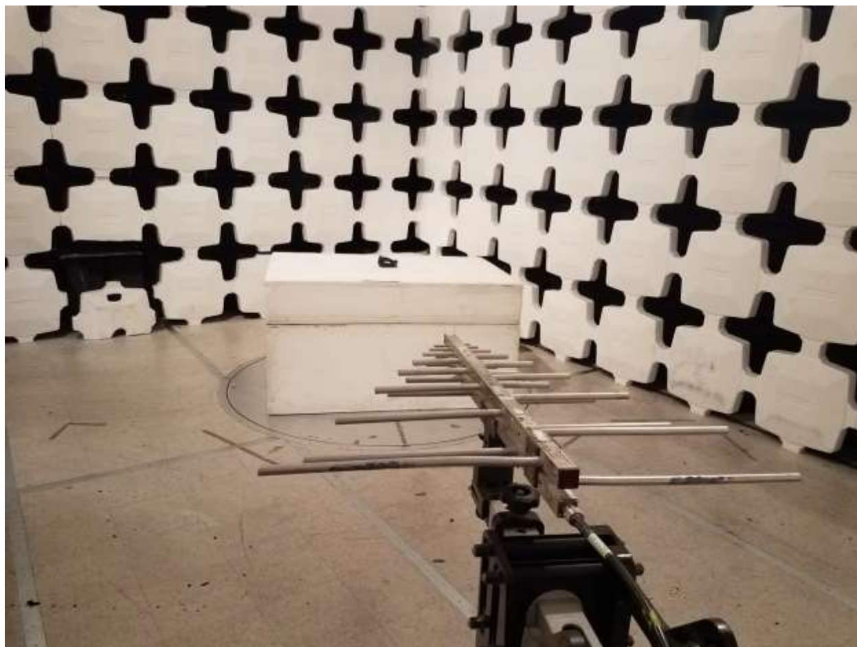
Figure 3. Radiated Emissions Test Configuration (200 MHz to 1 GHz) Intentional Emissions & Unintentional Emissions
