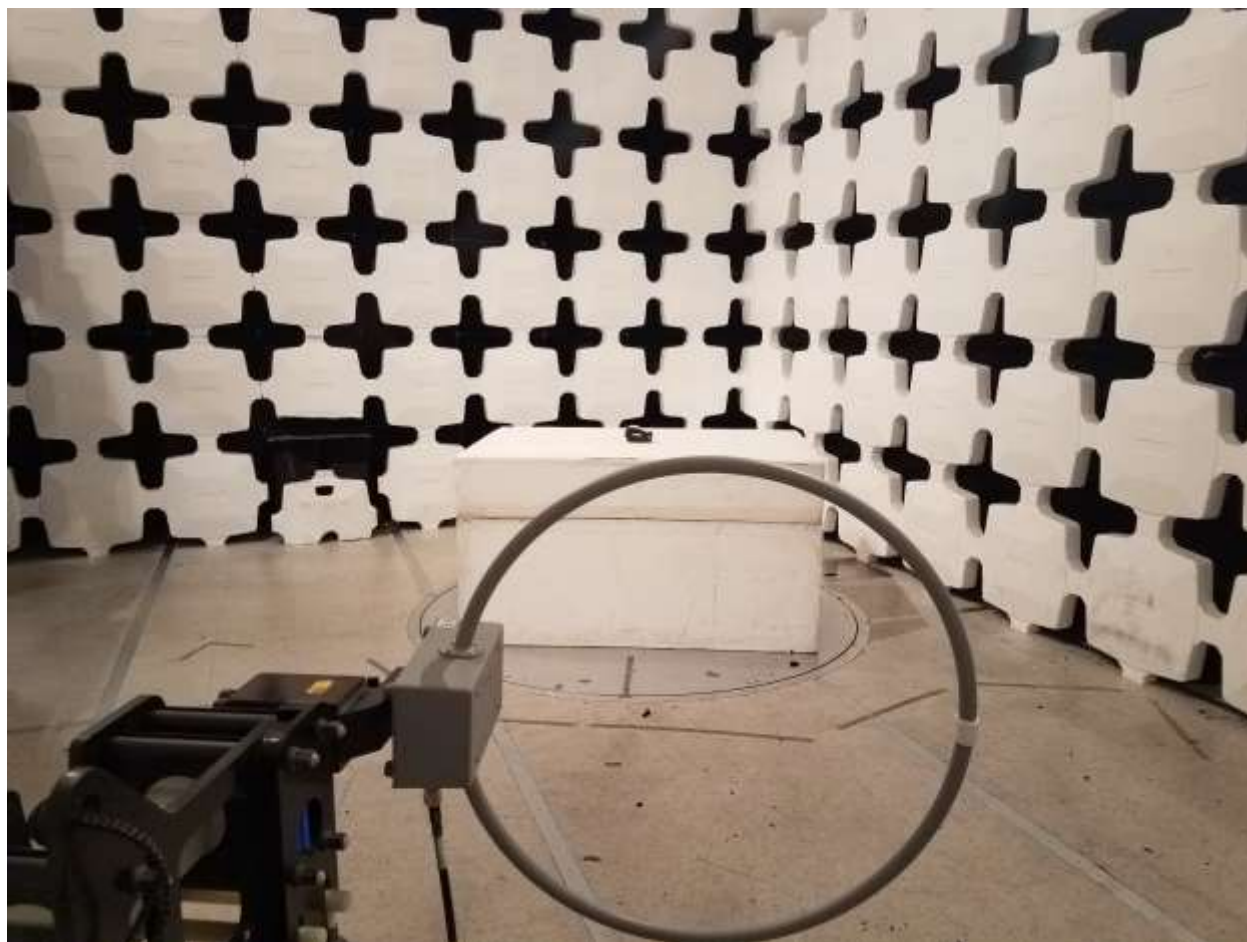
Figure 1. Radiated Emissions Test Configuration (Below 30 MHz)
