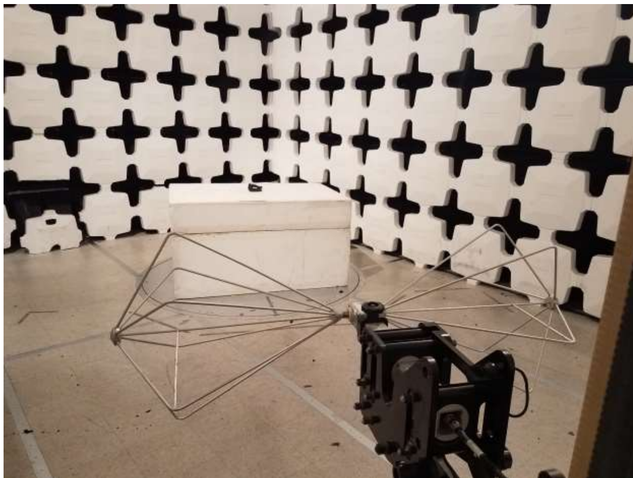
Figure 2. Radiated Emissions Test Configuration (30-200 MHz)
