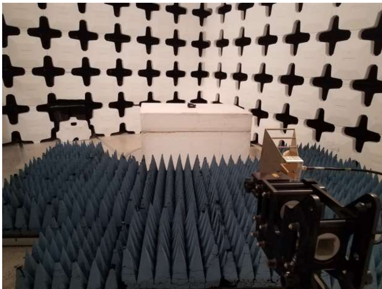
Figure 4. Radiated Emissions Test Configuration (> 1 GHz) Unintentional Emissions
